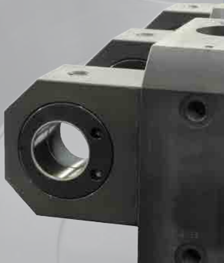
Example of microregulation of stroke on rear head bushing installed on cylinder 6020-2
