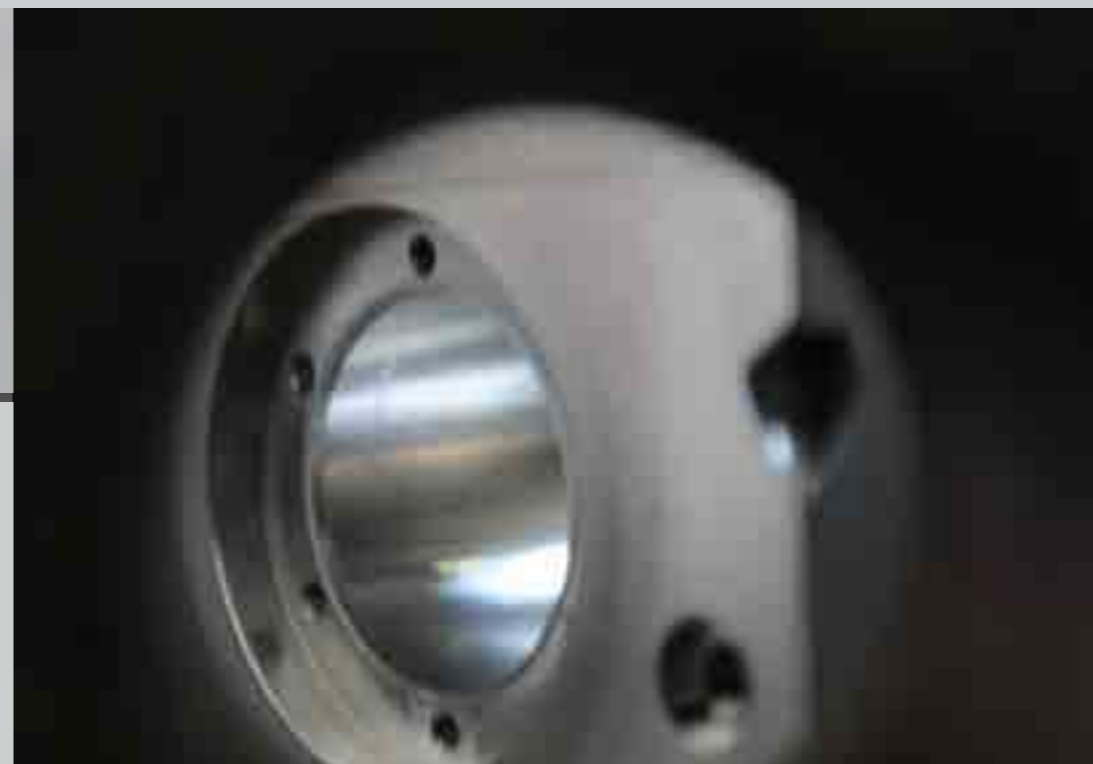
Example of external nitriding treatment on junction head
